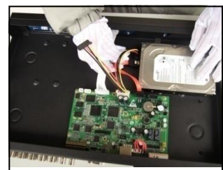
⑥ connect the power wire
