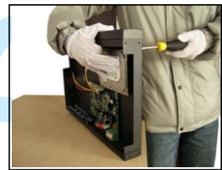
③ fix the screw of hard disk
