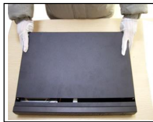
② disassemble the cover
