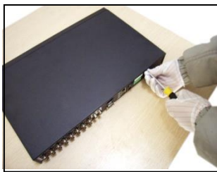
① disassemble the screw
