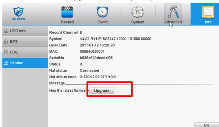
Click [Upgrade] button, the device will start to upgrade the new firmware, please do not power off & off network in the upgrade process
